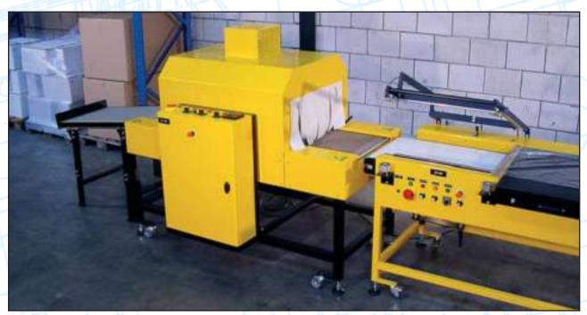
sistent high quality. Shrink tunnels are also designed with attention to the finest detail. For example, the air flow inside the tunnel can be adjusted by means of four valves inside the oven unit. Furthermore, the processing speed of the conveyor rollers is smoothly adjustable. The easily readable temperature is controlled and maintained
