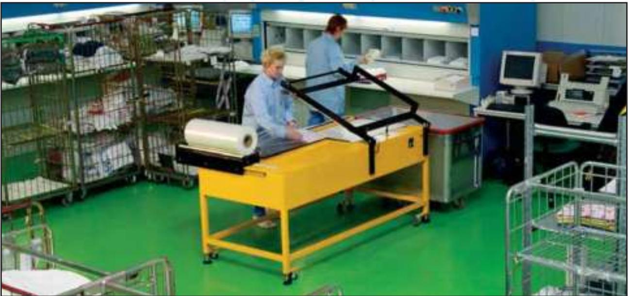
*Corner sealers can be seamlessly integrated into any production process, e.g. in a laundry as illustrated here.*
