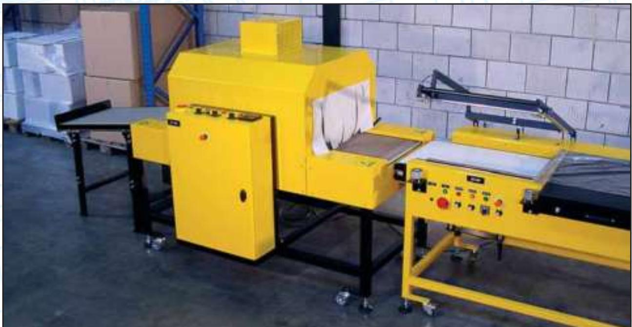
sistent high quality. Shrink tunnels are also designed with attention to the finest detail. For example, the air flow inside the tunnel can be adjusted by means of four valves inside the oven unit. Furthermore, the processing speed of the conveyor rollers is smoothly adjustable. The easily readable temperature is controlled and maintained
