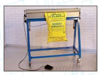
**SMS-IST** Super Magnet Sealers can be mounted on an industrial mobile work stand with height as well as angle adjustment.
